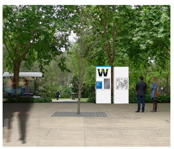
This sign must be integrated with tactile ground locators as specified in AS1428.4.1 Tactile Ground Surface Indicators.
